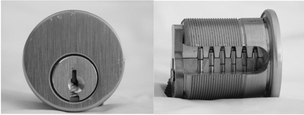
Figure 1: A pin tumbler lock cylinder. *Left*: The cylinder face. Note the *keyway*, which is cut into the *plug*, which in turn sits inside the *shell*. *Right*: Side view, with part of the shell and plug cut away to expose the six *pin stacks*. Note the border between the plug and shell, which forms the *shear line*, and the *cuts* in each pin stack resting within the plug.
