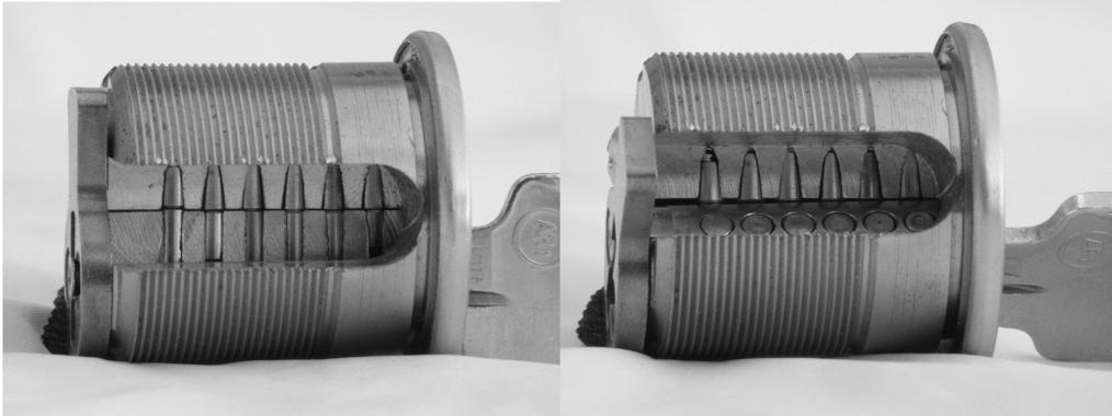
Figure 2: Pin tumbler lock with a correct key inserted. *Left:* The correct key lifts the pin stacks to align the cuts at the shear line. *Right:* With all of the cuts at the shear line, the plug can rotate freely within the shell. Here the plug has been turned slightly toward the camera, so that the tops of the pins in the plug are visible.
